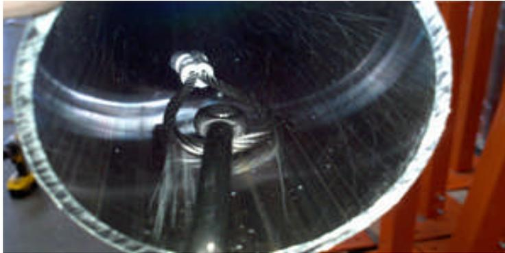
5. Screw the shackle pin through the inside and outside looped ends of the wire rope and tighten pin firmly.
