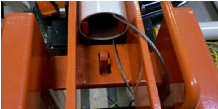
3. Unscrew and remove the shackle pin and slip the shackle on to the tube with the inside and outside looped ends of the wire rope aligned with the shackle hole drilled at the bottom of the tube.
