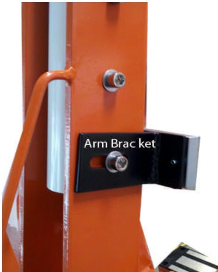
2. Pictured below is the magnet assembly for the arm-down magnetic lock. It is possible to adjust the arm up and down by loosening the adjustment bolt on each side and sliding the arm bracket up and down. Always try to maintain flat contact of both parts of the magnet assembly. The frame mounting bracket can be slid in and out to help line up the magnetic plates horizontally.
