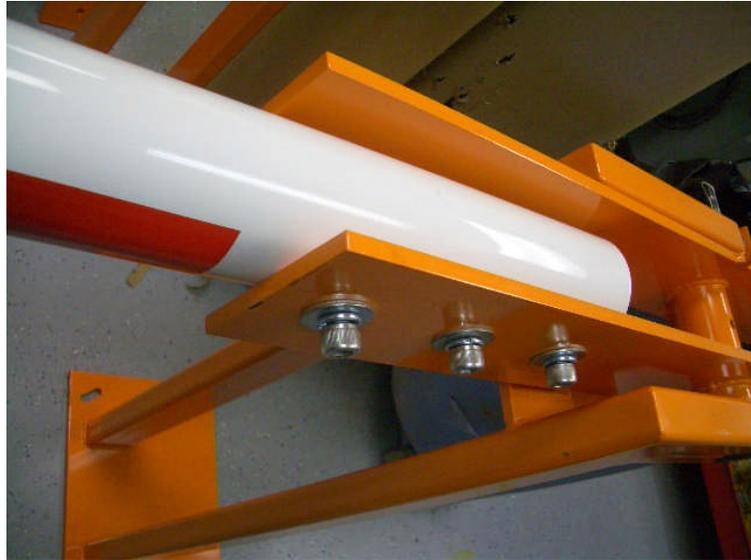
The picture above illustrates the arm bolted to the swing arm.
