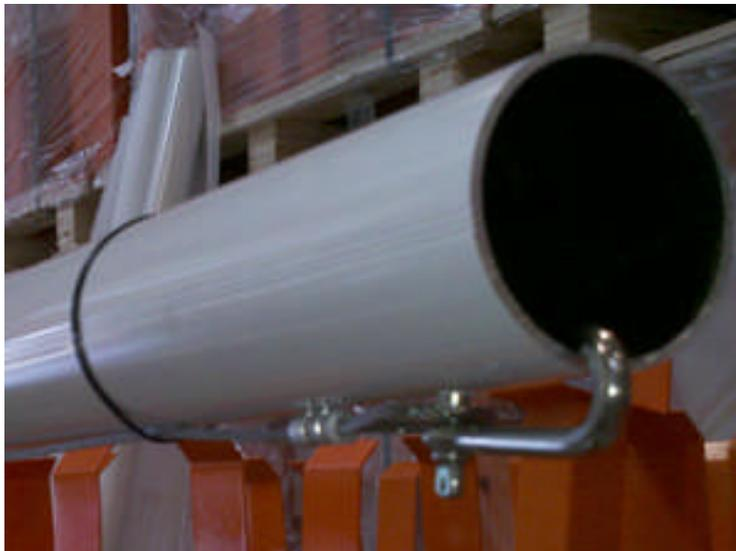
6. Drill a 3/8" hole in the plastic end cap to accommodate the shackle and tap the end cap back into place. Glue in with adhesive silicone if needed to secure cap.
